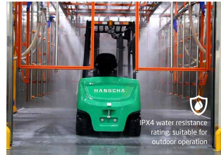
IPX4 water resistance rating, suitable for outdoor operation
