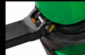
Pedestrian type use the new design drive system, the drive motor will not accompany the tiller rotation, it can keep all the cable connect to the drive motor avoid being bent.
