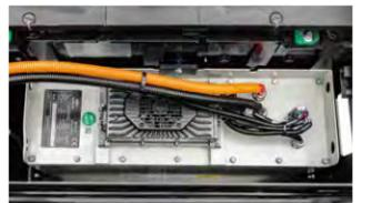
(Option) Lithium battery with the on-board charger (48V, 20A)
