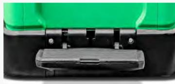
The standing driving pedal with shock-absorbing design significantly improves standing driving comfort and reduces long-time driving fatigue.
