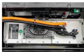
(Option) Lithium battery with the on-board charger(48V,20A)
