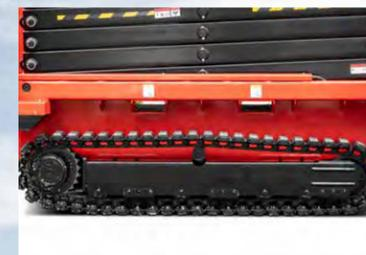
The protection class of traveling motor is IP67. Two-wheel drive, the combination of the permanent magnet synchronous motor and high-speed reducer make strong performance.
