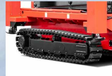
The machine is moving by the crawler, it has high friction coefficient and high driving strength. Fully sealed permanent magnet synchronous drive motor, it makes fast walking speed, strong power and high efficiency.
