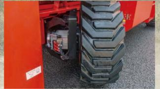
Permanent magnet motor drive, energy efficient, more powerful, excellent waterproofing grade IP67.
