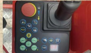
Portable drive box integrates drive and lift and one button leveling function, The steering control is arranged at the end of the handle, so that the single handle can flexibly control the travelling speed , steering function and lifting height of fence.
