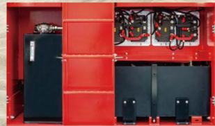
Large capacity lithium iron phosphate battery, combined with two groups of large capacity cell lithium iron phosphate, the total capacity of 19kWh. The vehicle is equipped with backup power supply for safety emergency descent. In case of equipment failure or other sudden situations when operators are working at heights, they can switch emergency operations to lower the equipment to the lowest place.
