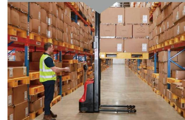
With the remote control device, you can easily set the speed suitable for the work, from level 1 speed to level 5 speed. Such speed transitions allow you to move the truck with controlled operation at ease.
