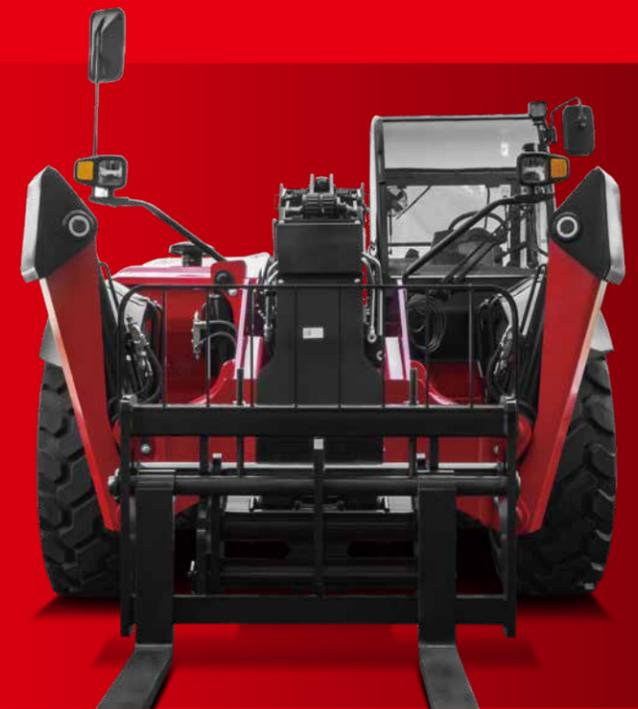
With efficient operation performance, the maximum speed is 35 km/h, the maximum climbing ability is 40%, and the lifting height is industry-leading in the same category.
