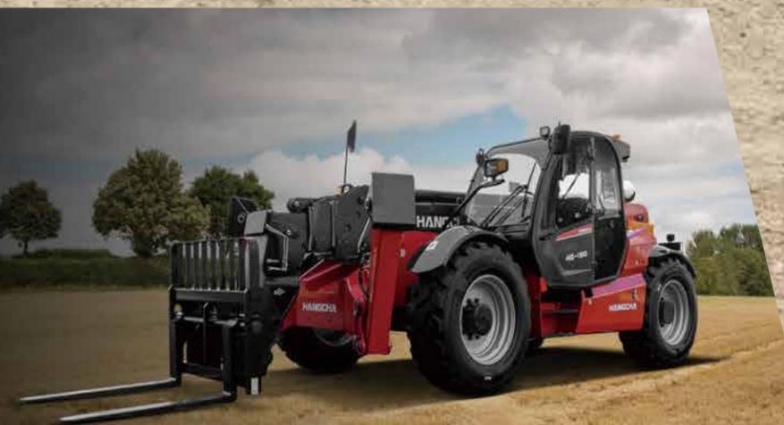
The machine is equipped with quick change device, which can realize the quick replacement of different attachments. This enables various operations including fork loading, shovel loading, clamping, aerial work, etc.
