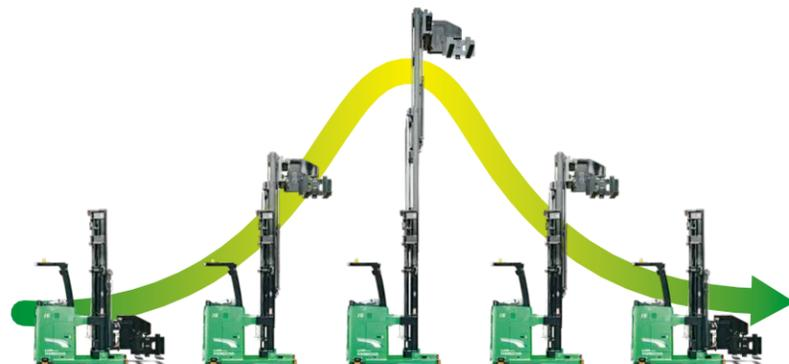
The oil pump motor assembly is provided on the rear side of the stacker, so that the center of gravity of the whole stacker moves backwards and the stability is better.
