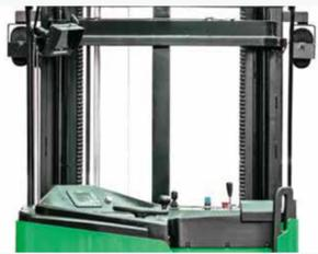
The new design of the mast structure enables the stacker to have an excellent operating view and to access the pallet more easily.
