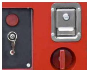
Manual lowering handle, When the operation system failed or the battery power is too low to let the platform decline, we can use this handle to lower the machine
