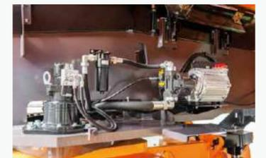
Permanent magnet motor drive variable piston pump, strong performance and low energy consumption.
