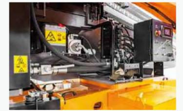
With the 12V emergency power system, the operator can be safely returned to the ground even if the main battery is out of power.
