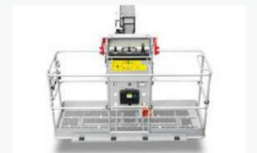
2.44 m large basket, can accommodate 3 people working at the same time. The basket controller is equipped with 3 proportional control handles, and the boom expansion and amplitude variation support simultaneous movements.
